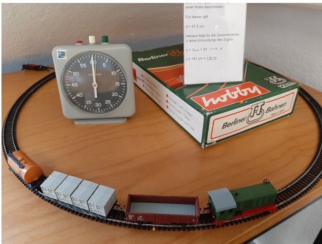
FIG. 1: Entire equipment of the experiment containing a clock and a train on rails (voltage source excluded being below the table).
