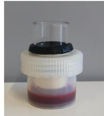
Figure 5 Fully assembled *in vitro* feeding chamber, containing bovine blood.
